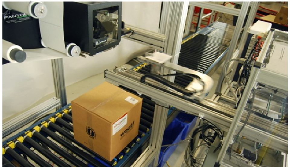
Full size packing sheet is automatically printed, "folded & tucked" under the removable shipping label as shown below.
