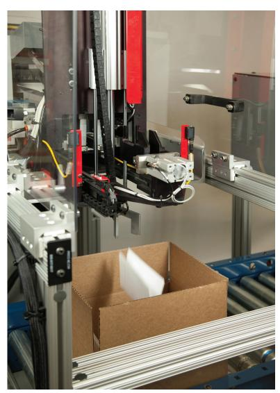
PFI™ carton height detection automates the placement of the document based on the carton height. The unit accurately prints, folds, and places one to ten 8.5″ x 11″ printed sheets into cartons ranging from 4″ to 30″ in height.
